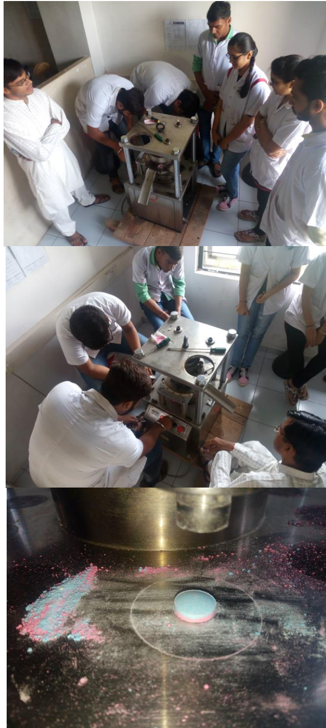
B. Pharm. Students themselves setting punches and dyes, and operating the Rotary Tablet Punching Machine, preparing bilayered tablets
